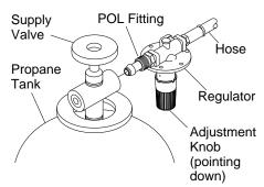
Figure 3 - Regulator With Adjustment Knob Pointing Down
